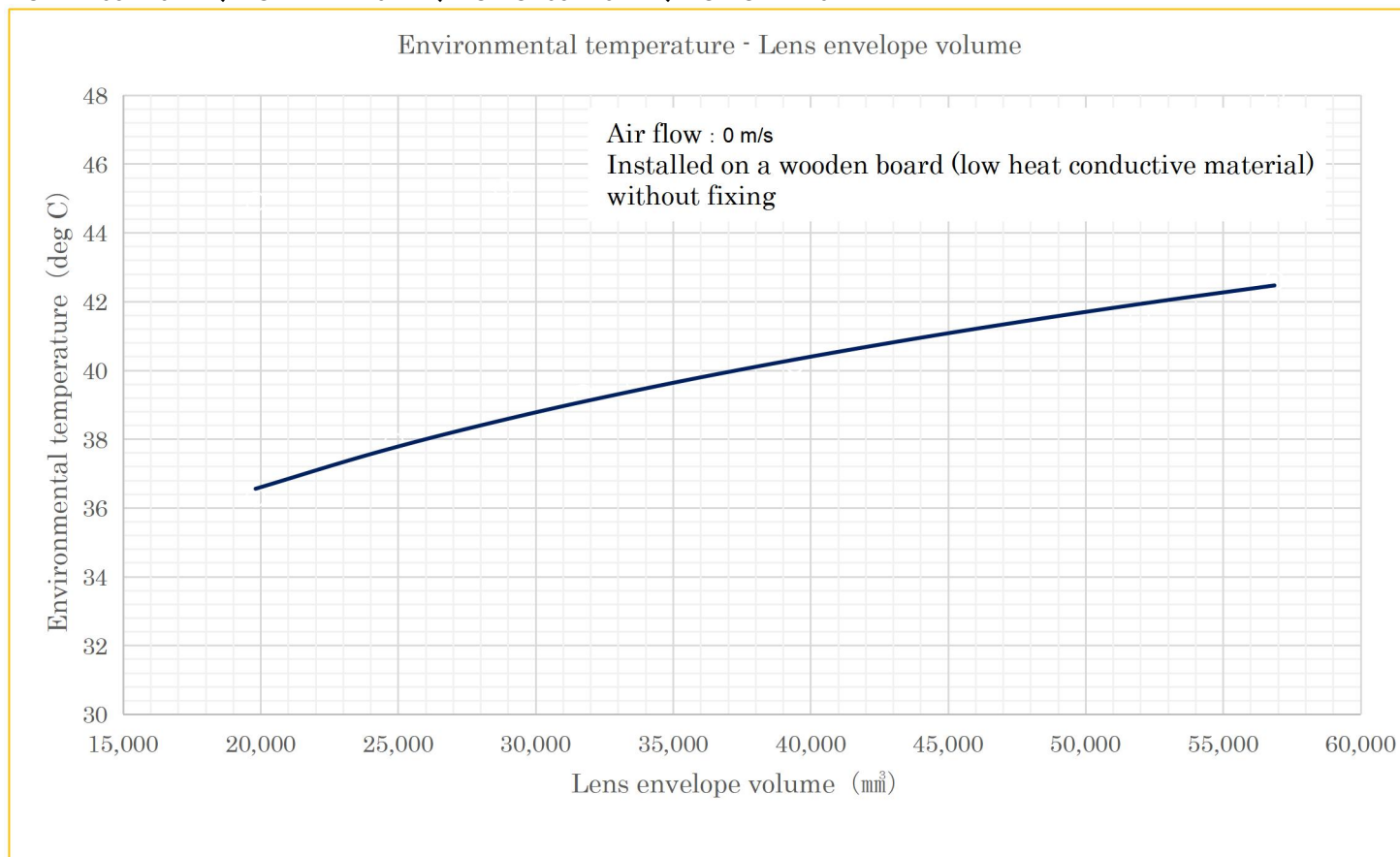
(Reference) Fig1.3-2 Relationship between attached lens size and usable environmental temperature (Camera installation : Worst condition、 Device Temp.=70 deg C)
