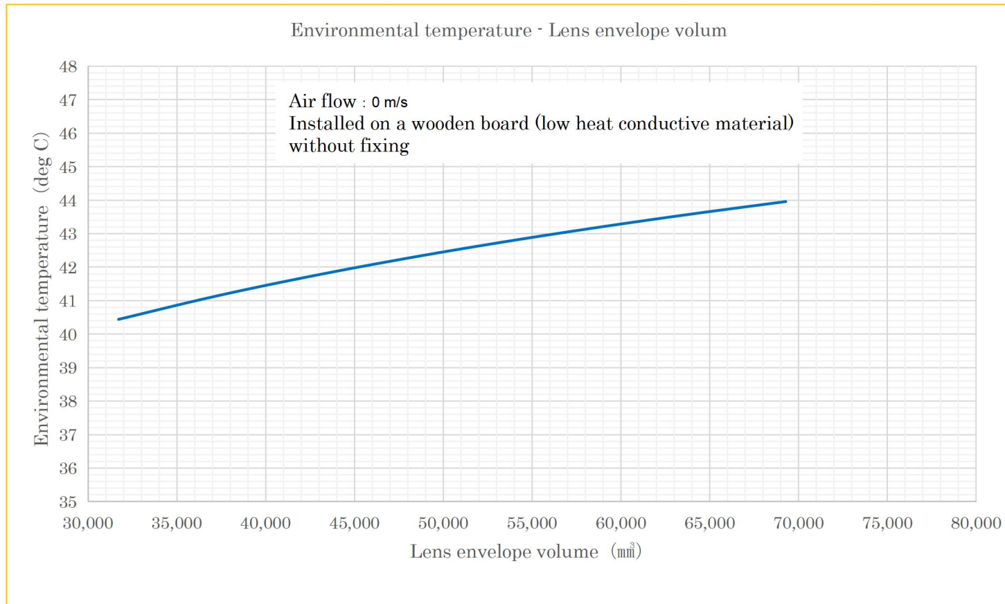
(Reference) Fig1.3-3 Relationship between attached lens size and usable environmental temperature (Camera installation : Worst condition、 Device Temp.=70 deg C)
