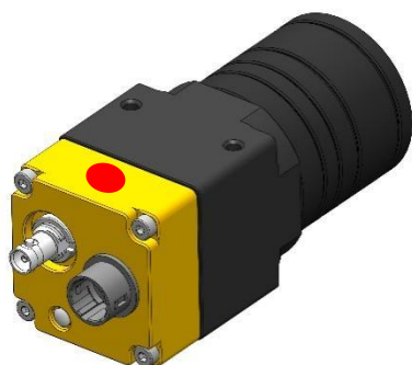
Fig1.3-1 Camera housing measuring point
