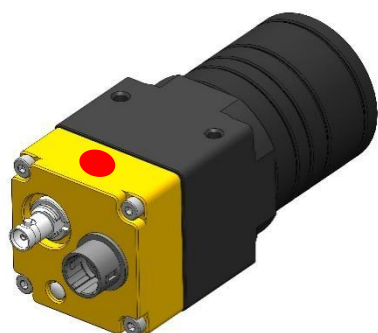
Fig1.3-1 Camera housing measuring point
